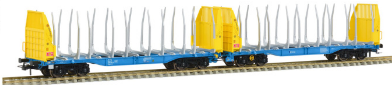
S657111 CD Cargo articulated double timber transport wagon Sggmrrs | CD Cargo Doppel Holztransportwagen Sggmrrs - A-IF 35 81 4657 010-8
