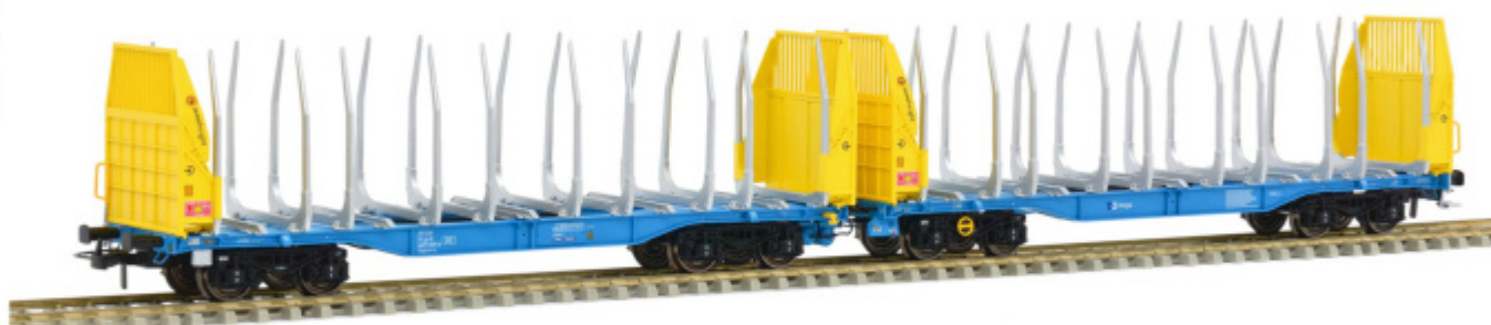
S657009 CD Cargo articulated double timber transport wagon Sggmrrs | CD Cargo Doppel Holztransportwagen Sggmrrs - A-IF 35 81 4657 009-0
