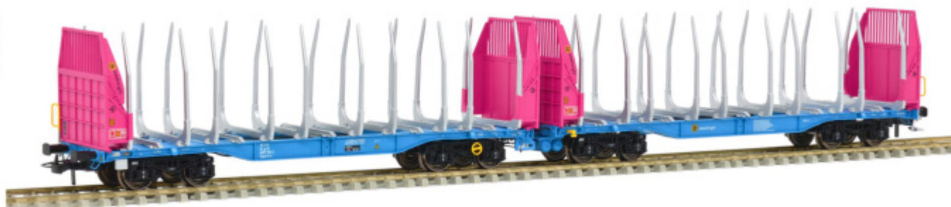
S657319 Innofreight articulated double timber transport wagon Sggmrrs | Innofreight Doppel Holztransportwagen Sggmrrs - A-IF 35 81 4657 319-3
