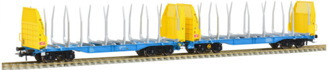
S657095 Innofreight articulated double timber transport wagon Sggmrrs | Innofreight Doppel Holztransportwagen Sggmrrs - A-IF 35 81 4657 095-9
